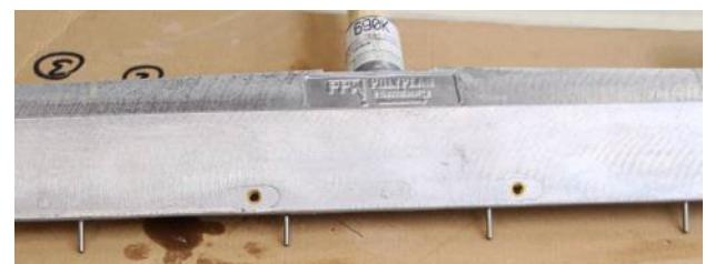
The pin squeegee must be set [1-2mm](#) higher than the desired thickness of the elastic layer.
