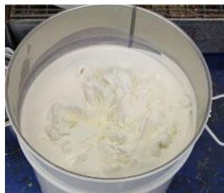
Then component [B](#) is poured into component [A](#). Make sure, that the pail, containing component [B](#) is emptied completely.
